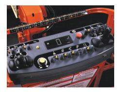
**Ground Control Console.** Ground control console features a three-dimensional decal. A detailed light panel provides status of specified machine conditions, including various self-diagnostic maintenance sensors. Ground control console is conveniently located at eye level for ease of use.
