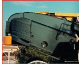
Interactive counter-weight system covers range of boom angles
